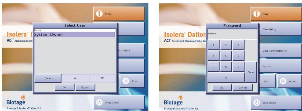
Figure 2-1. Log into the Data Administration Mode (Isolera Dalton 2000 System with Assist Workflow Enabled Shown)
