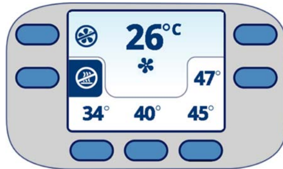
Figure 4-5. Warming System Set to Heat Off
