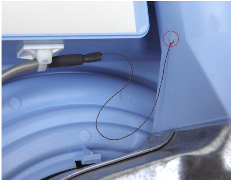
Figure 11-2. Thermistor Wire and Rivet
