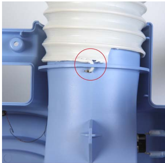
Figure 11-20. Wire Attaching Hose to Hose Duct Adapter
