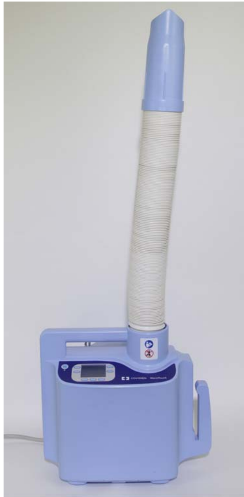
Figure 7-4. Position of Hose for Temperature Accuracy Test
