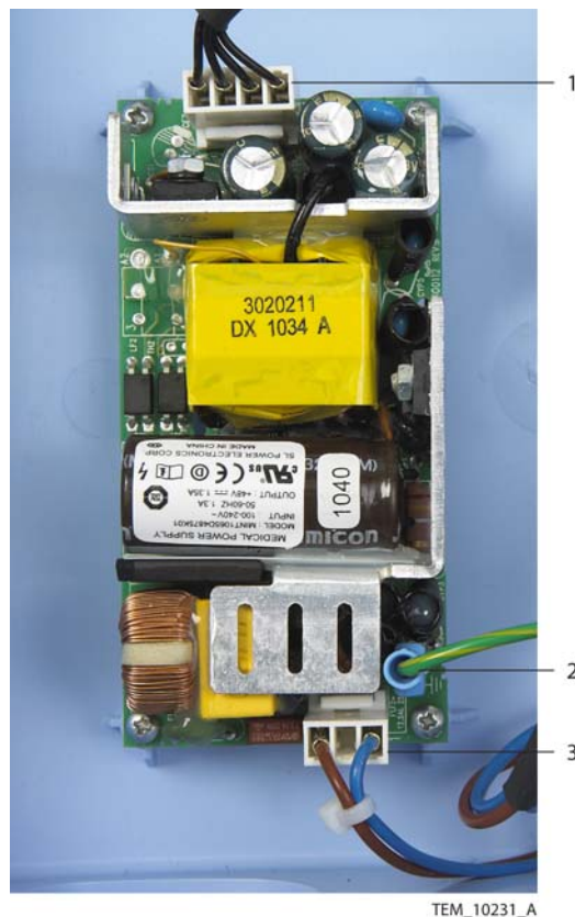
Figure 10-32. Power Supply Connections
