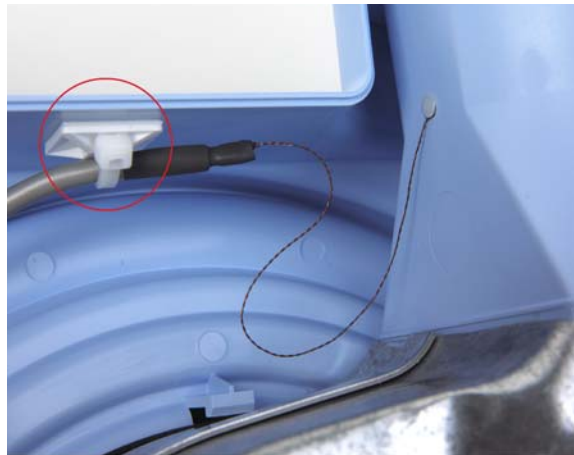
Figure 12-28. Thermistor Cable Secured
