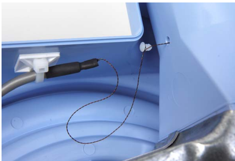
Figure 11-29. Inserting Thermistor Wire and Rivet
