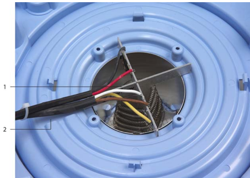
Figure 12-23. Routing of Heater Wires
