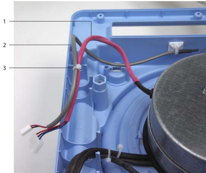
Figure 11-35. Cable Tie Securing Fan Cable to Thermistor Cable
