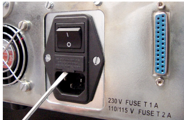
Figure 4-8. Loosening the Hinged Fuse Holder Cover
